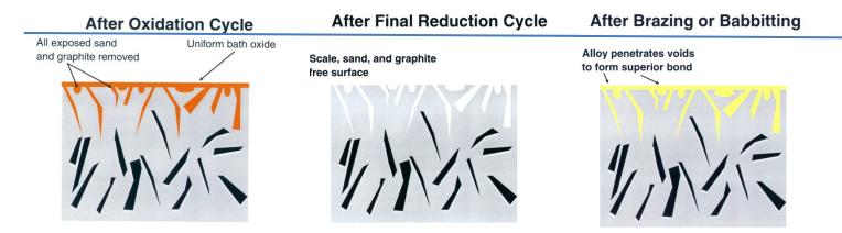
A final reversal of the casting's polarity to negative or reducing results in a casting surface that is chemically-cleaned and free of scale, sand, and graphite and ready for brazing, joining, or coating operations (above middle).
